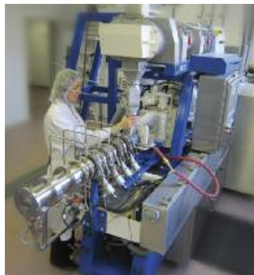
The twin screw extruder at the Food Centre has helped them explore opportunities in high moisture protein fibrillation.
